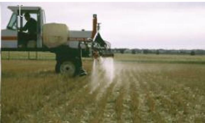
Figure 3. Air induction nozzles at 70 psi. (Wolf)
